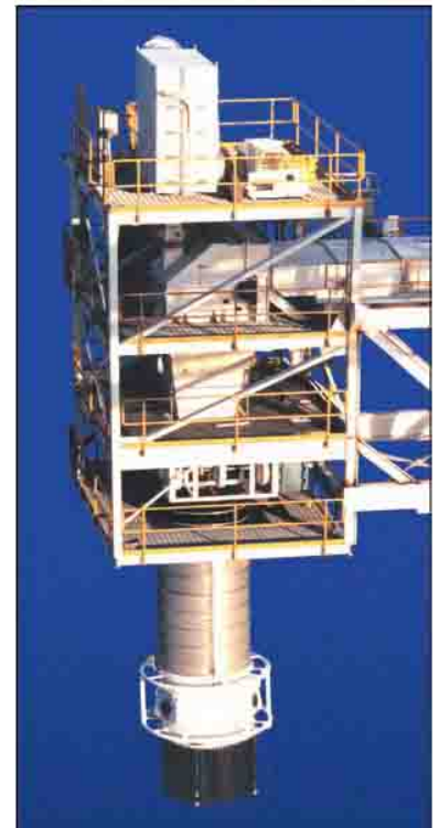
Unique OV66HD with 100 feet of travel loading extremely dusty kaolin clay.
