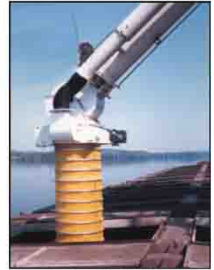
Pivoting gimbal allows different loading angles.
