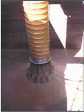
Dust free grain loading into barges.
