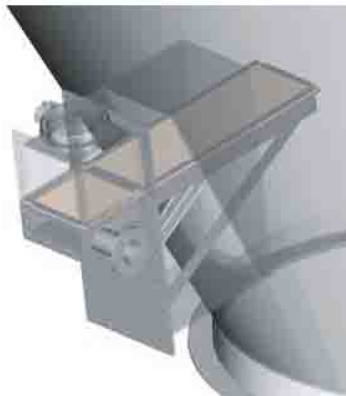
Aeration conveyor being fed by bucket elevator.
