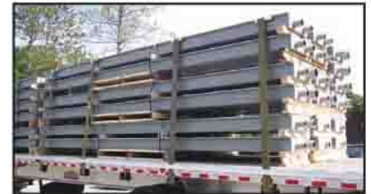
Aerated troughs for dome floor installation.
